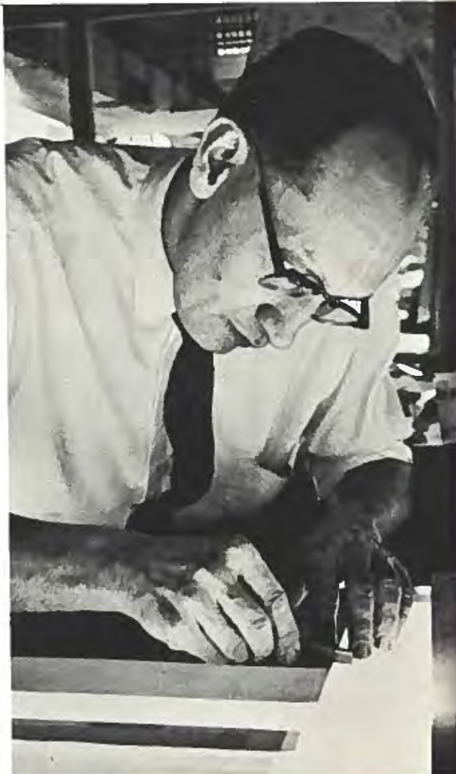
At the Wm. J. Keller plant in Buffalo, Beck makes three-color pre-separations to match the dummy by placing black strips on large clear acetate sheets.
